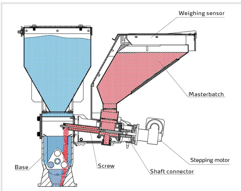
Signals from control cabinet are sent to motor, then motor begins to work, the rotary force is transferred to dosing screw through shaft connector. Masterbatch in hopper falls into the groove of conveying screw, and then be taken to hopper base by rotating action of the screw. Weighing sensor is adopted to precisely control masterbatch output to fulfill proportional adding.
